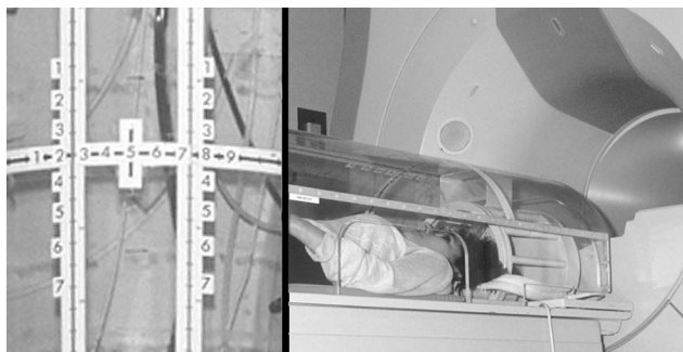
FIGURE 1. Left: detail of fixation device with numbered fixation marks; Right: subject on dolly in front of MR scanner bore, with fixation device in place and adjusted to proper distance from globes.
