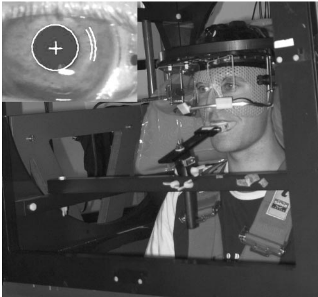
FIGURE 1. Photograph of the setup with the eye-movement recording devices. A subject who is held in place with a bite bar wears the Chronos head device and is surrounded by a cubic frame that contains the field coils. The inset shows an image, recorded and used by the Chronos recording and analysis software, of a subject's eye with scleral search coil inserted (partially visible around the limbus). Also shown is the fit through the pupil ( white circle ) and its center position ( white cross ), as well as an iris signature with two segments ( curved white lines to the right of the pupil).
