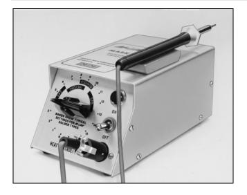
A time-proven precision soldering instrument for miniature and/or delicate soldering applications. Full 25-watt rating in 17 selector positions to handle all M-LINE solder alloys except 1240-FPA. Magnetic solder pencil holder and flexible, burn-resistant cord. Lightweight soldering pencil (1.1 oz [31 g]). Specify 115 or 220 Vac, 50 or 60 Hz operation.
